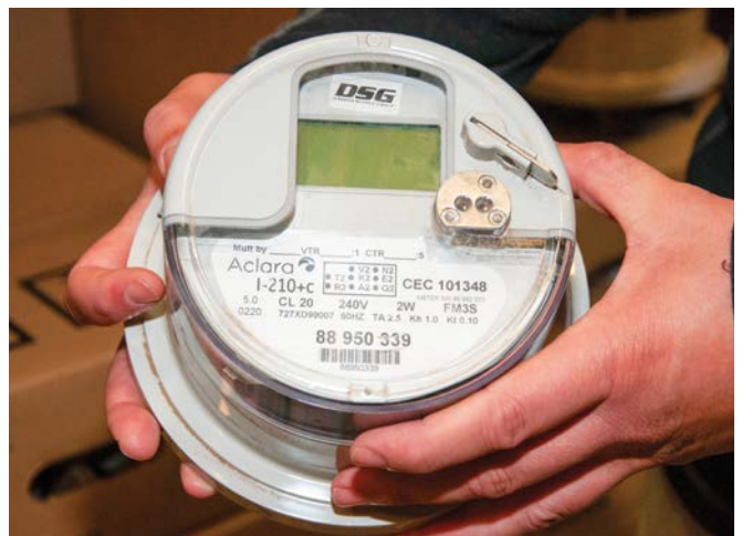
Over the next three years, Capital Electric Cooperative will complete the final phase of its meter system upgrade, replacing old meters with wireless cellular meters. The new metering system provides fast, two-way, real-time communication with the co-op's control room. Once the transition is complete, it will allow the control room and dispatchers to have a near real-time view of the entire system.
