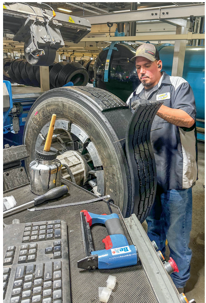
Ramon demonstrates the most important step in the process, the application of the new tread. Using the most recent technology creates a high-quality product. Ramon completes the process of sealing the tread prior to curing.
